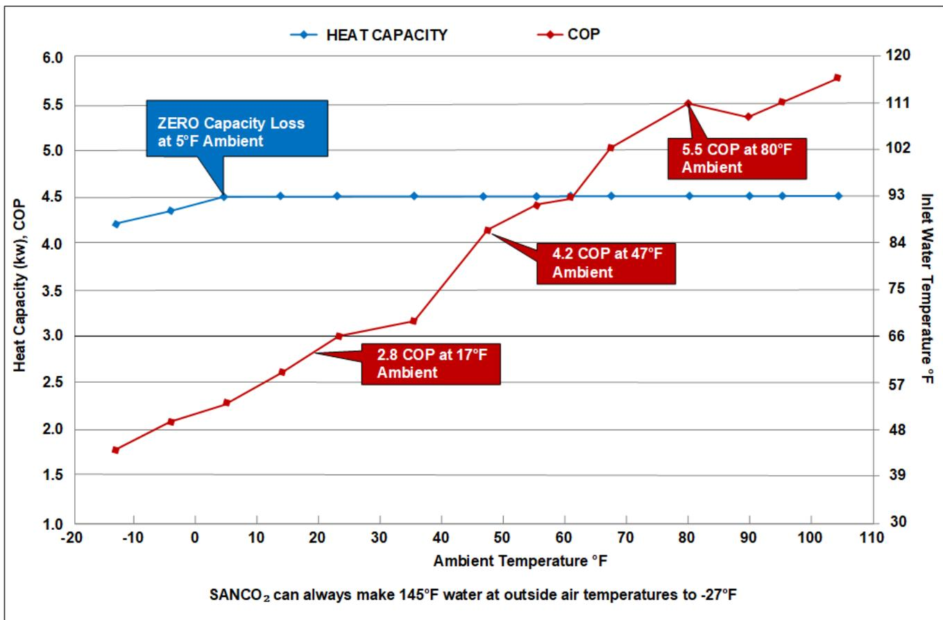
As can be seen, at 5°F ambient the system COP is over 2.0, which rises to over 4.0 at 47°F ambient, rising to 5.0 at 67°F ambient and 5.5 at 80°F ambient
