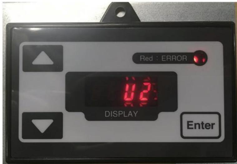
After a component is replaced or the inspection is completed, turn the breaker OFF for a period of 3 minutes before restarting to confirm the error does not reoccur.
